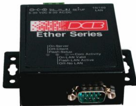
Figure 3 - Example of SCADA device
